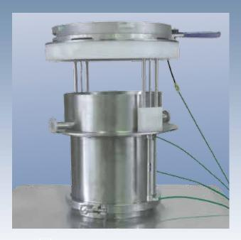
The METO Systems FIBC Docking System has an integrated iris valve that provides material flow control, and an inflatable seal system ensures a contained transfer of product. The optional dust extraction system provides additional dust control for applications requiring higher containment of the product.
